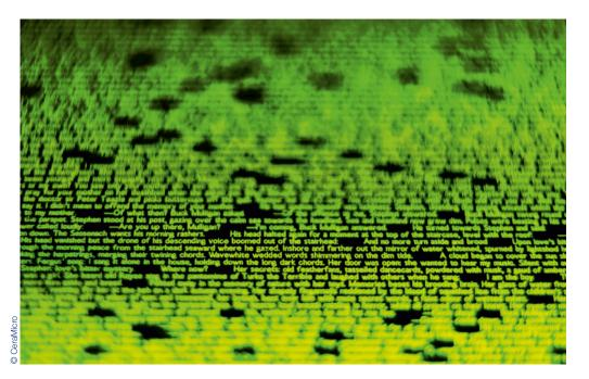
ceramic carrier. Five million characters fit onto a 200 mm x 200 mm panel of ceramic microfilm. Two such panels suffice to save all of the Harry Potter volumes for posterity. Patents protect the concept of a durable ceramic data carrier.
