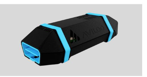
test driver through the test procedure. The analysis uses data that provide information on features such as voltage, power and temperature. The enormous amount of data is transmitted to the backend at Aviloo by mobile phone, where machine learning algorithms are used to determine the battery's "health".
